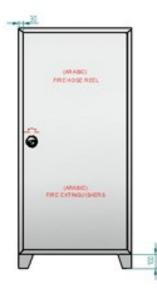
Cabinets are manufactured from Stainless steel a thickness of 0.9mm to 2mm thick which depens on usage or customer requist.
