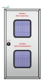
Cabinets are manufactured from Stainless steel a thickness of 0.9mm to 2mm thick which depens on usage or customer requist 6MM Wired glass installed in the door.
