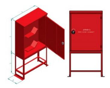
Cabinets are manufactured from Mild steel a thickness of 0.9mm to 2mm thick which depens on usage or customer requist. Leg height as per customer requirement. Standard Leg height is 600mm Cabinets are painted with Powder Coated for elegant finish and protection from rust
