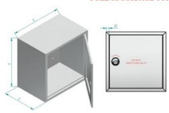
Cabinets are manufactured from Stainless steel a thickness of 0.9mm to 2mm thick which depens on usage or customer requist
