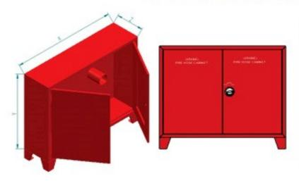
Cabinets are manufactured from Mild steel a thickness of 0.9mm to 2mm thick which depens on usage or customer requist. Leg height as per customer requirement. Standard Leg height is 100mm Cabinets are painted with Powder Coated for elegant finish and protection from rust
